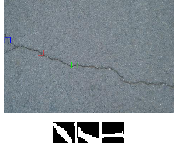
Fig. 6. Assigning y to each image patch. The image patches have been assigned to the tokens below respectively (both from left to right).
